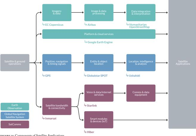
FIGURE 12: Components of Satellite Applications
