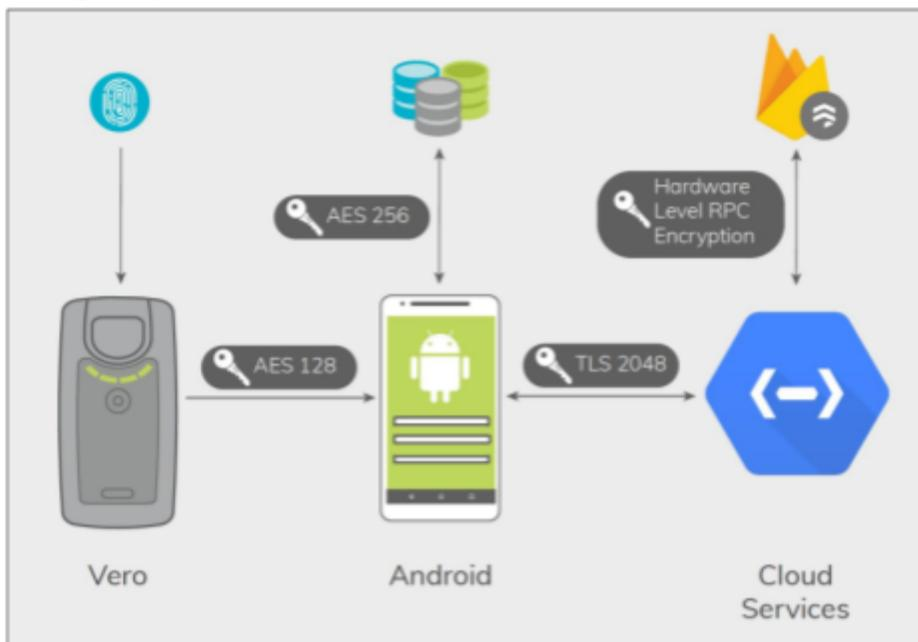
Figure 9: Simprints System Architecture for one fingerprint reader system with encryption between data points [credit: simprints]
