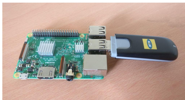
Figure 1: RASP-IVR is a low cost ($50) IVR system consisting of a Raspberry Pi and a GSM modem.
